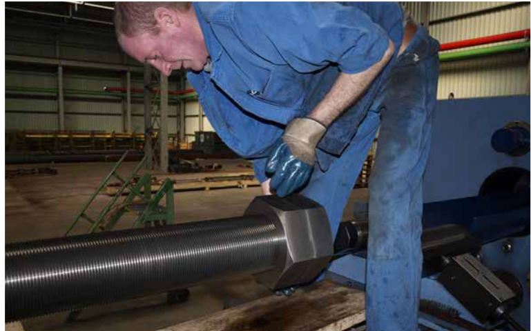
M160x6 Offshore foundation (Malaysia)
