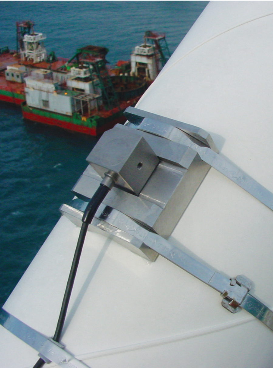
Stay cable fitted with an accelerometer
