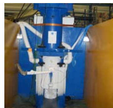
Cryogenic test on Freyssinet C-system
